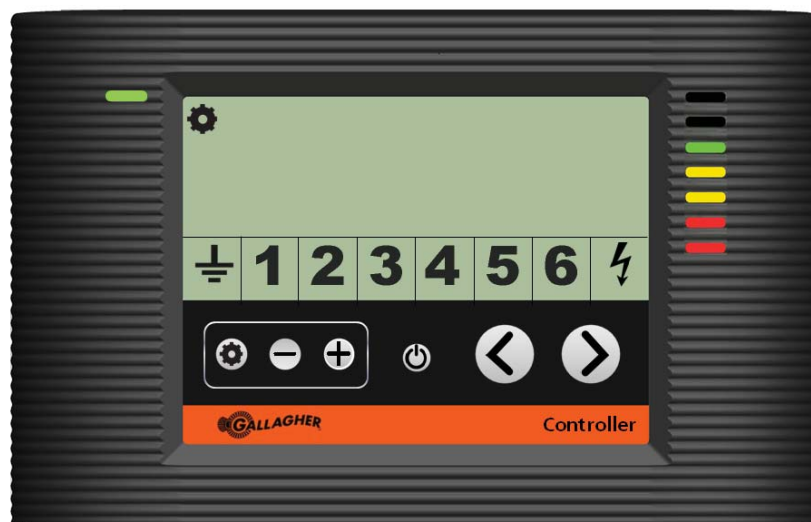
Controller showing the output voltage being adjusted
