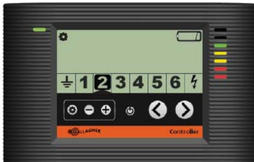
Bedieningspaneel toont zone 2 met lege batterijen
